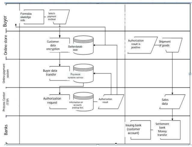
Fig. 1.The process of operations of e-commerce system with the participation of TTP
